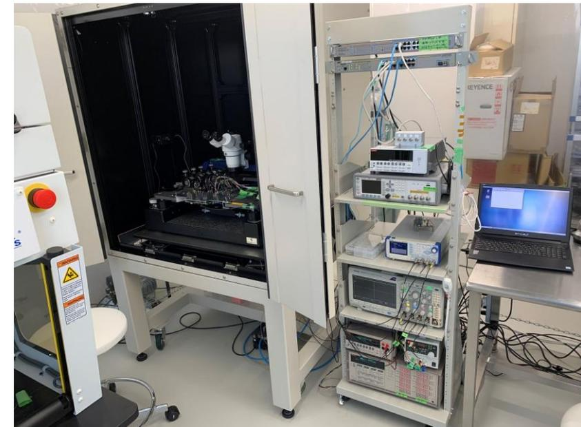
Probe station and measuring devices
