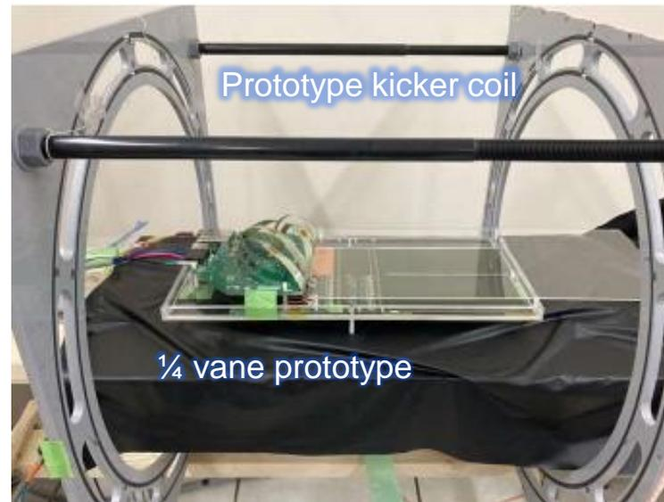
Operation test in kicker magnetic field at Tokai
