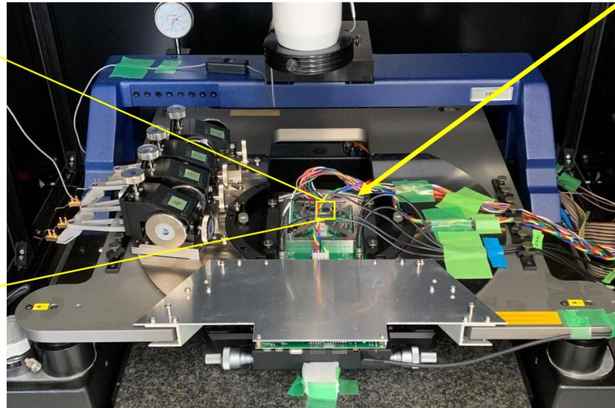
Probe station with probe card installation
