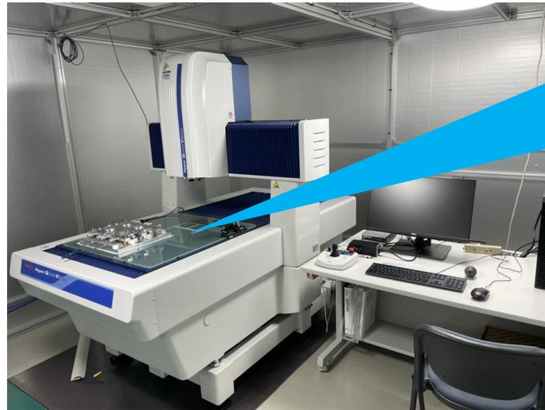
3D coordinate measuring machine at KEK
