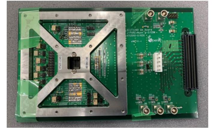
Probe card for readout ASIC
