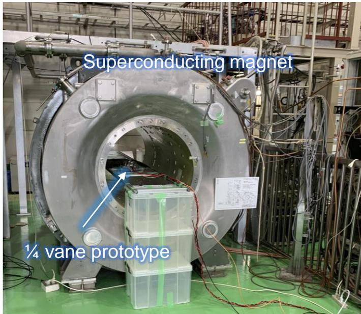
Operation test in high magnetic field at KEK
