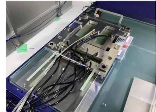
Assembling jig for readout boards
