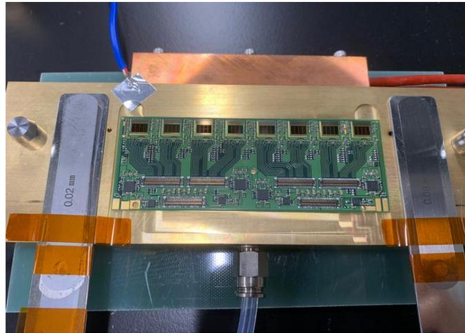
Circuit board on assembling jig
